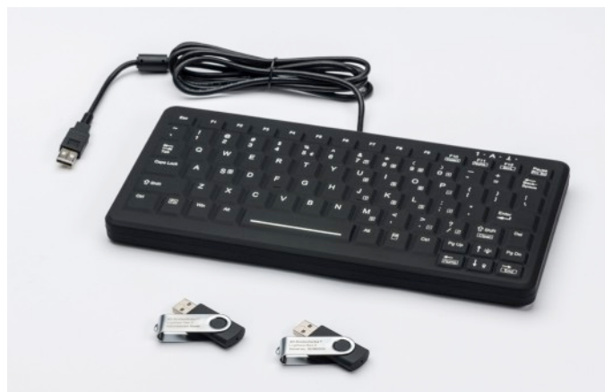
Components of the 4D-Nucleofector® LogWare Gen 2: USB Sticks for LogWare installation and administrator reset and supportive external keyboard
